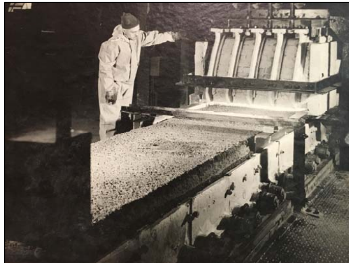
Figure 26. Muffle for igniting charge on Dwight Lloyd Sintering Machines, 1930s.
