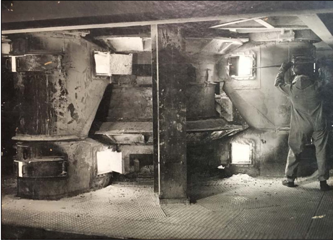
Figure 30. Blowing air into the oxide furnace with tuyeres, 1930s. 83
