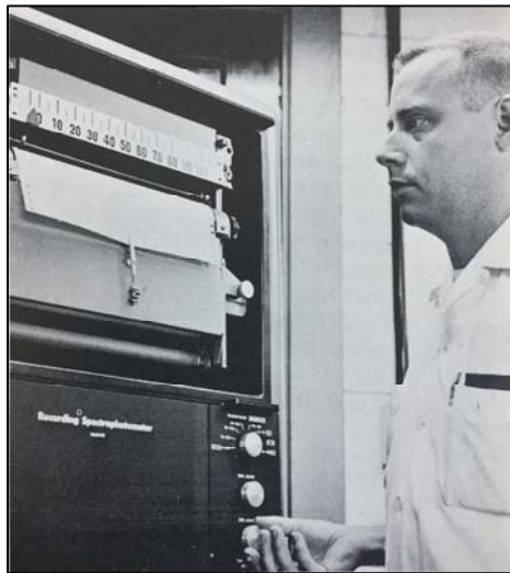
Figure 58. Chemist operating the research spectrophotometer measuring zinc oxide color, 1960. 218
