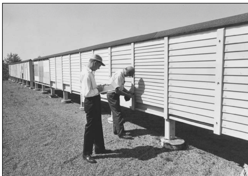
Figure 57. Paint lab's sampler for paints made with St. Joe oxide. 210
