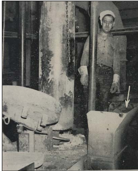
Figure 62. Ira Sullivan at furnace chute, 1946. He suggested this chute to improve cleaning out of condenser down-legs in the furnace. 248
