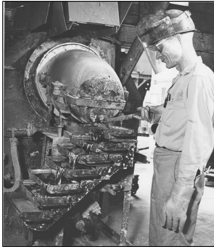
Figure 17. Pouring cadmium in the leach plant, constructed in 1937. 48
