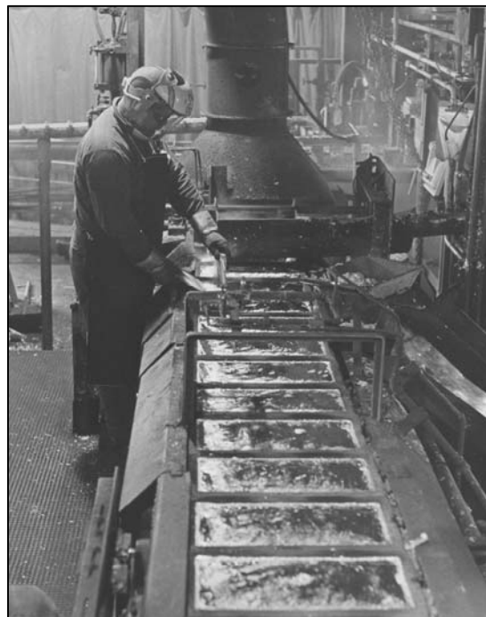
Figure 29. Casting zinc metal, c. 1964. 82
