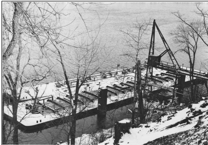
Figure 25. Loading sulfuric acid into a barge for transport on the Ohio River. Acid was also shipped in tank trucks and tank railroad cars. 69
