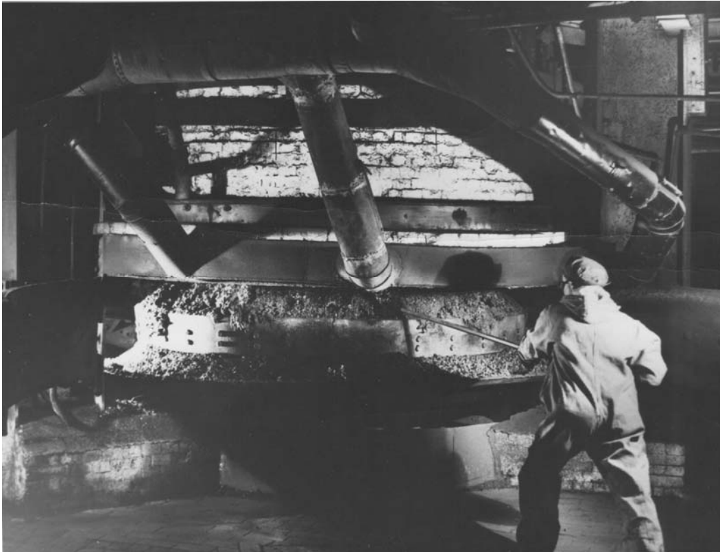
Figure 18. Residue from the furnace tables worked with hand-bars before the “Cam-O-Tactor,” 1930s. 56
