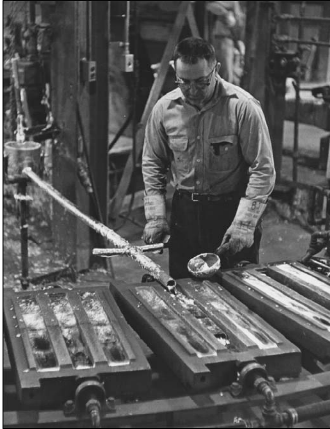
Figure 31. Pouring zinc anodes in the refinery. 86
