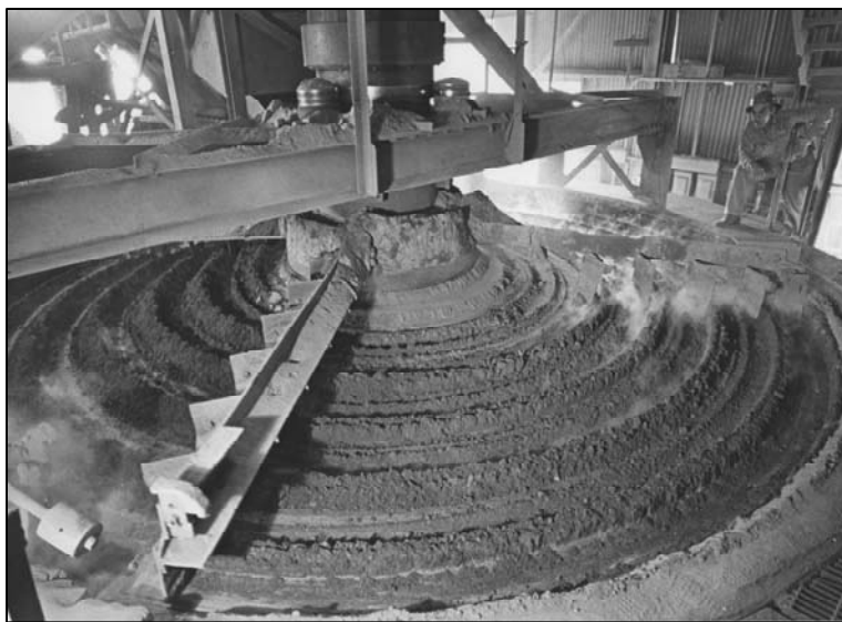
Figure 23. Drying hearth in the hearth roaster. 62
