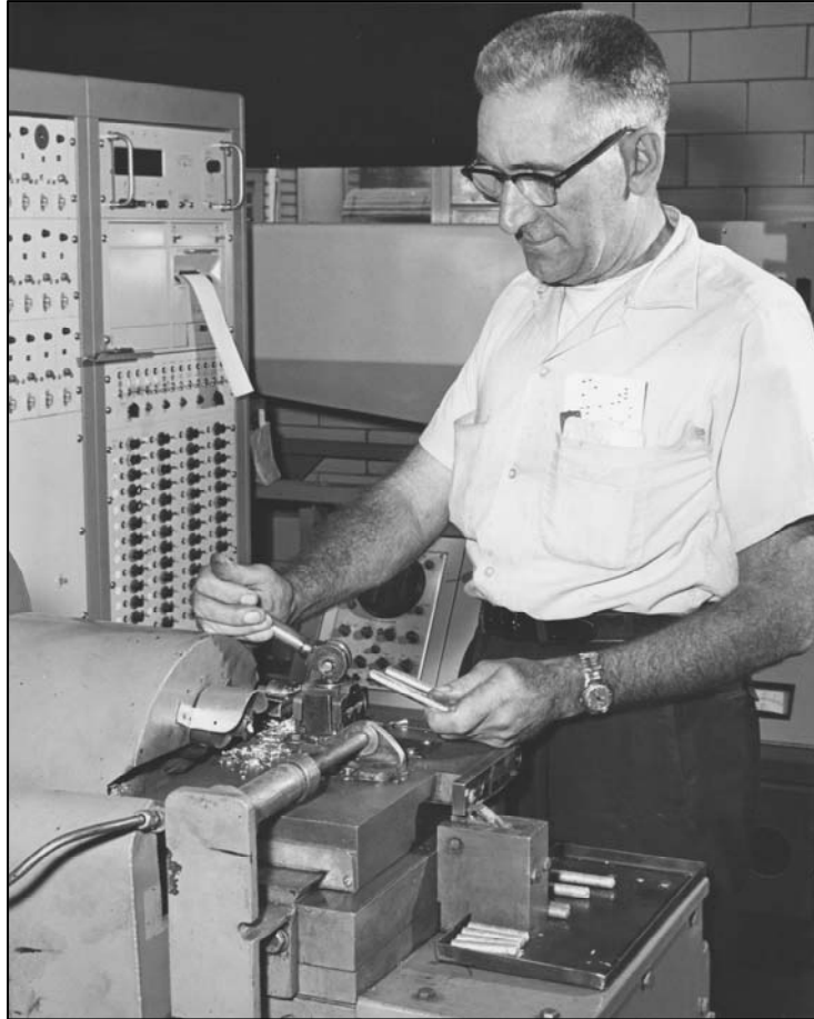
Figure 43. Pin shaper in Direct Reader Spectrometry Laboratory. Used to prepare zinc pins for sampling content. 124
