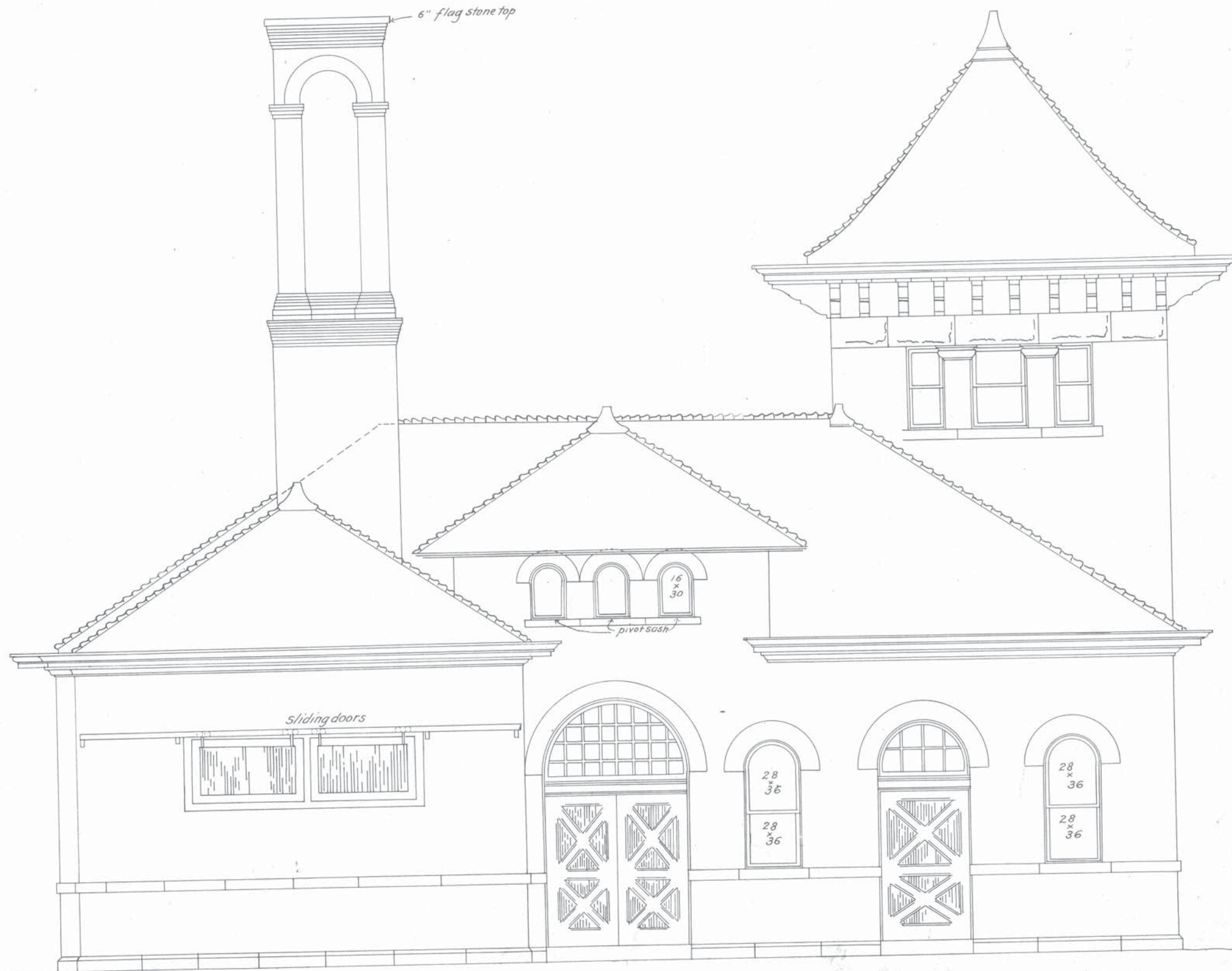
RAILROAD ELEVATION SCALE \frac{1}{4} " = 1 FOOT. POWER HOUSE FOR LOCK No. 6: OHIO RIVER. DRAWN BY DIRECTION OF W. E. GRAIGHILL CAPTAIN, CORPS OF ENGINEERS U.S.A.
