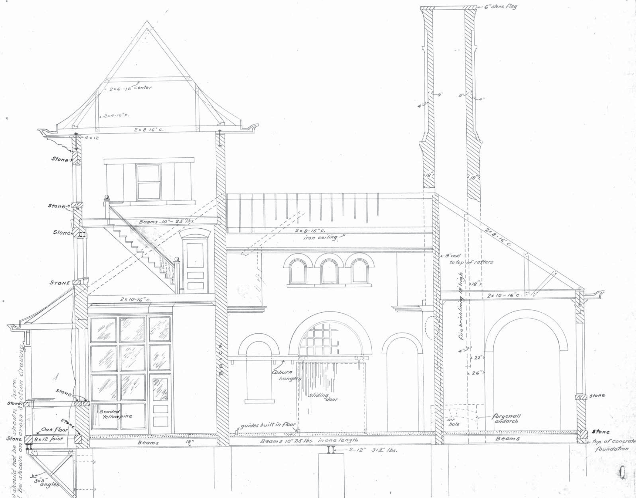
LONGITUDINAL SECTION. SCALE \frac{1}{4}'' = 1 \text{ FOOT} POWER HOUSE FOR LOCK NO. 6: OHIO RIVER DRAWN BY DIRECTION OF W. E. GRAIGHILL CAPTAIN, CORPS OF ENGINEERS, U.S.A.
