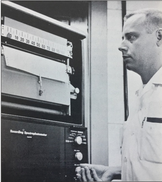
Figure 33. Chemist operating the research spectrophotometer to measure zinc oxide color, 1960.
