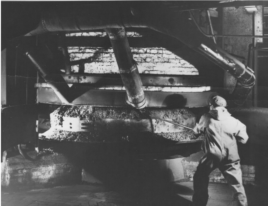
Figure 21. Residue from the furnace tables worked with hand-bars before the “Cam-O-Tactor,” 1930s.
