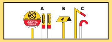
Line markers also identify the pipeline operator, the product transported and an emergency phone number.
